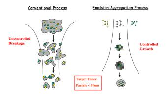
Figure 1. EA vs conventional process for making toner particles.
