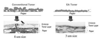
Figure 4. Thinner toner layer on substrate enabled by smaller *EA* toner.
