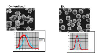
Figure 2. Particle shapes and distributions produced by EA and conventional processes.
